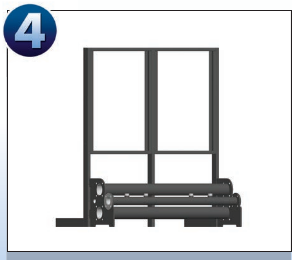
Step 4: Fit boiler frames
