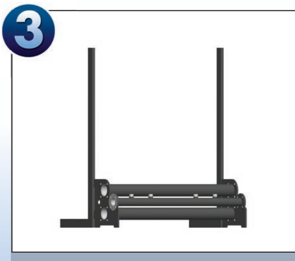
Step 3: Fit 'L' or 'I' support frames
